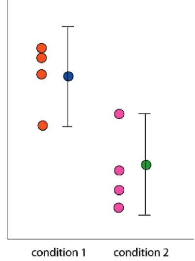
If the error bars for two measurements overlap, then we cannot conclude that the values are truly different.
