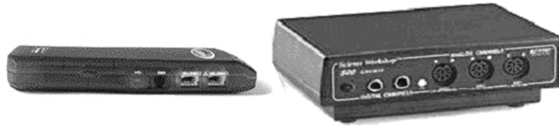
Figure 8.10 Analog-to-digital converters from Vernier and Pasco. Either box connects to the computer's serial port. A variety of probes can be connected to the box's front (shown).
