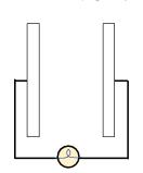
3. Plates remain connected and bulb goes out.
