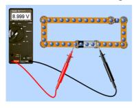
We can measure voltage differences with a **voltmeter** (as shown on the left). The voltmeter has a black and a red lead. To find out the voltage difference between two points on a circuit, put one lead on one point and the other lead on the other point. The voltmeter cannot be part of the circuit for it to work.
